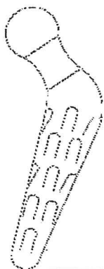
The diagram shows an artificial hip joint. When it is cooled the teeth lie flat and allow it to be inserted into the top of the thighbone.
